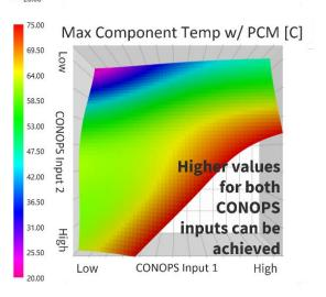
Momentus needed to finalize a thermal design that balanced temperature and energy requirements within a complex multi-dimensional design space. One example was interest in reducing battery temperature and minimizing required heater power. While battery mounting options with high conductance values help reduce battery temperature in the hot-case, they also require more heater power to maintain temperature in the cold-case.
